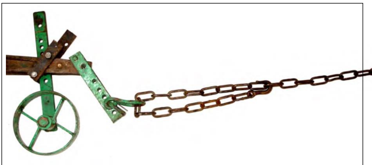
Figure 24: Trek chain with a hook at the end to easily adjust for effective chain length (Courtesy of GART 2004)
