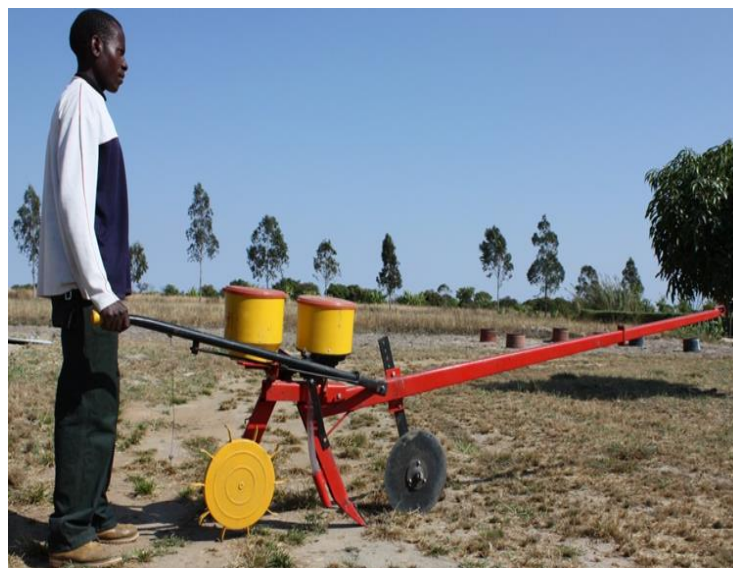
Figure 29: The Fiterelli direct planter and fertiliser applicator
